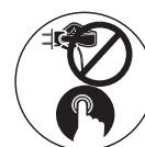
Don't pull wire to unplug machine, switch off & catch the plug and pull out.
