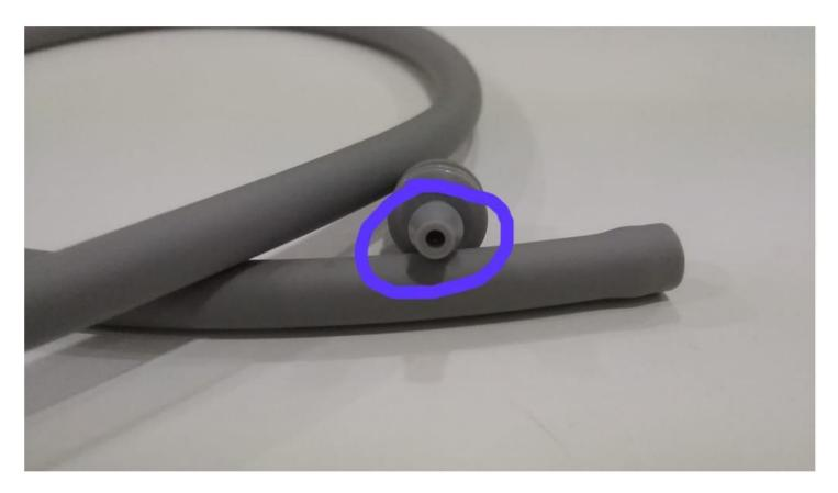
• After removing glue from tip of the nozzle hole you put it again in to tube and then check your Error - 5 will be solved.
