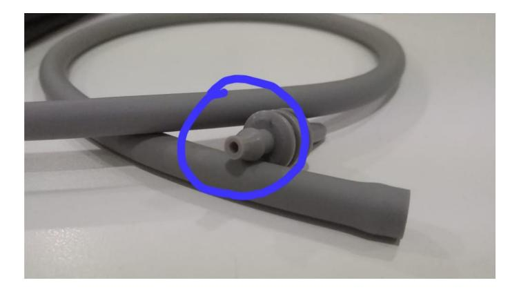
• After removing nozzle check this hole, there may me solution on that hole that you can easily remove with your finger nail or with sharp object.
