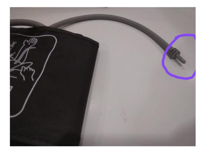
• First try to push air through this nozzle with mouth if cuff gets air and it goes proper then there is no issue in nozzle. If air is not getting in through this nozzle, then you have to remove this nozzle
